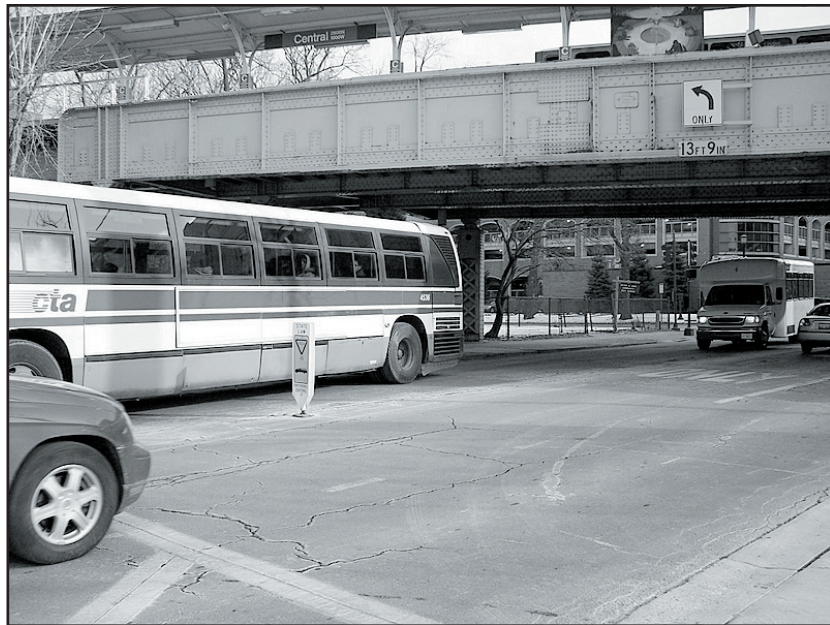
The presence of a turning lane, bus stops, and cars dropping off commuters results in congestion at the CTA station near Girard Avenue.
